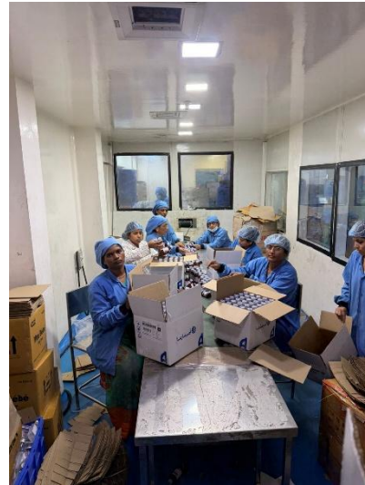
Packaging of liquid dosage forms (syrops) including bottle filling and carton packing.
