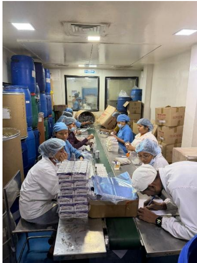
Packaging of solid dosage forms (tablets) using blister packing and labelling processes.
